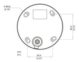
Figure 10.2: Dimensions - Mounting Holes
