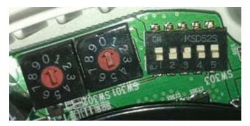
Figure 6.3: Close-up of Rotary Switches and Dip Switches
